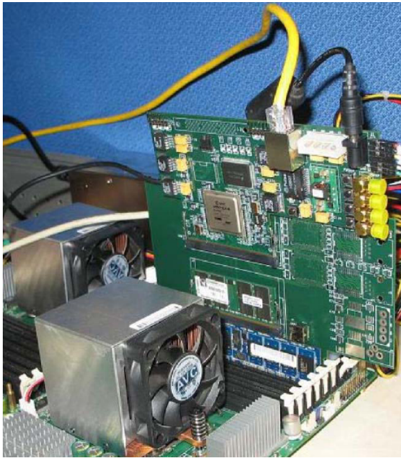
Fig. 8. The HMTT Tracing System. It is plugged into a DIMM slot of the traced machine. The main memory of the traced system is plugged into the DIMM slot integrated on the HMTT system.
