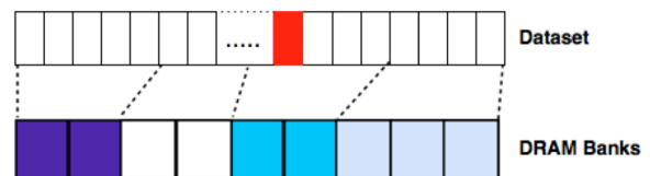
Figure 6: Thread Level Coloring. The above array is mapped to different bank colors. The colored rectangle in dataset represents shared data.
