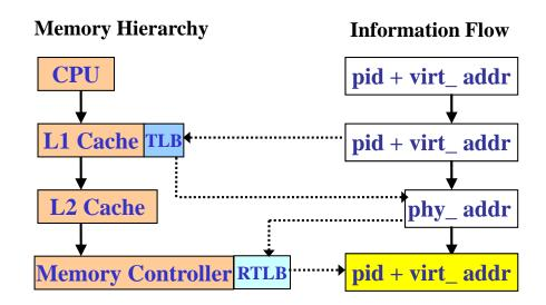
Reverse-TLB (RTLB) is introduced to support virtual channel mechanism for memory controller design, avoiding cache and program codes modification.
