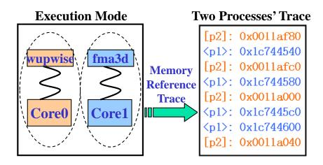
Physical addresses are interleaved among multiple processes. Most proposed optimization techniques at memory controller level use only the interleaved addresses, and may not achieve same improvements in multicore platform, because they cannot differentiate address spaces of VMMs/processes.
